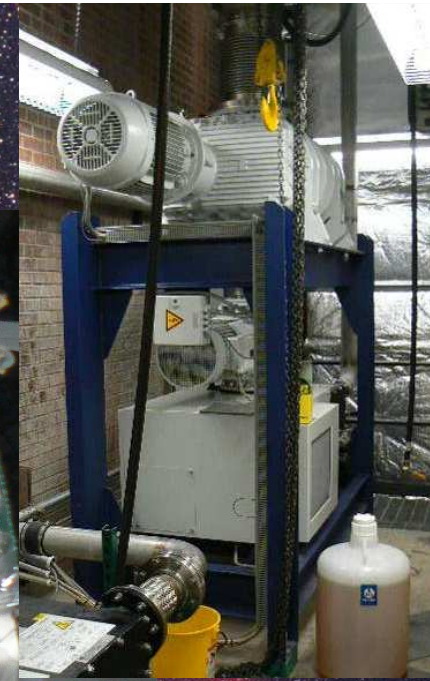
High-throughput Roots pump for future use of supersonic discharge source
