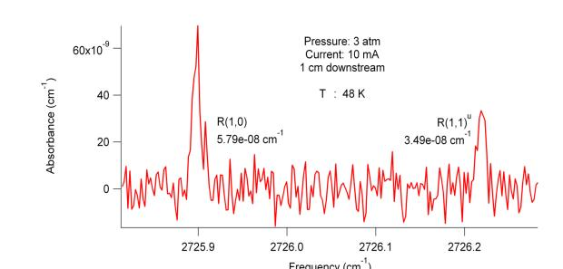
Spectra were also obtained after varying the current from 10 to 130 mA. It was observed that as the current increased, the signal increased.
