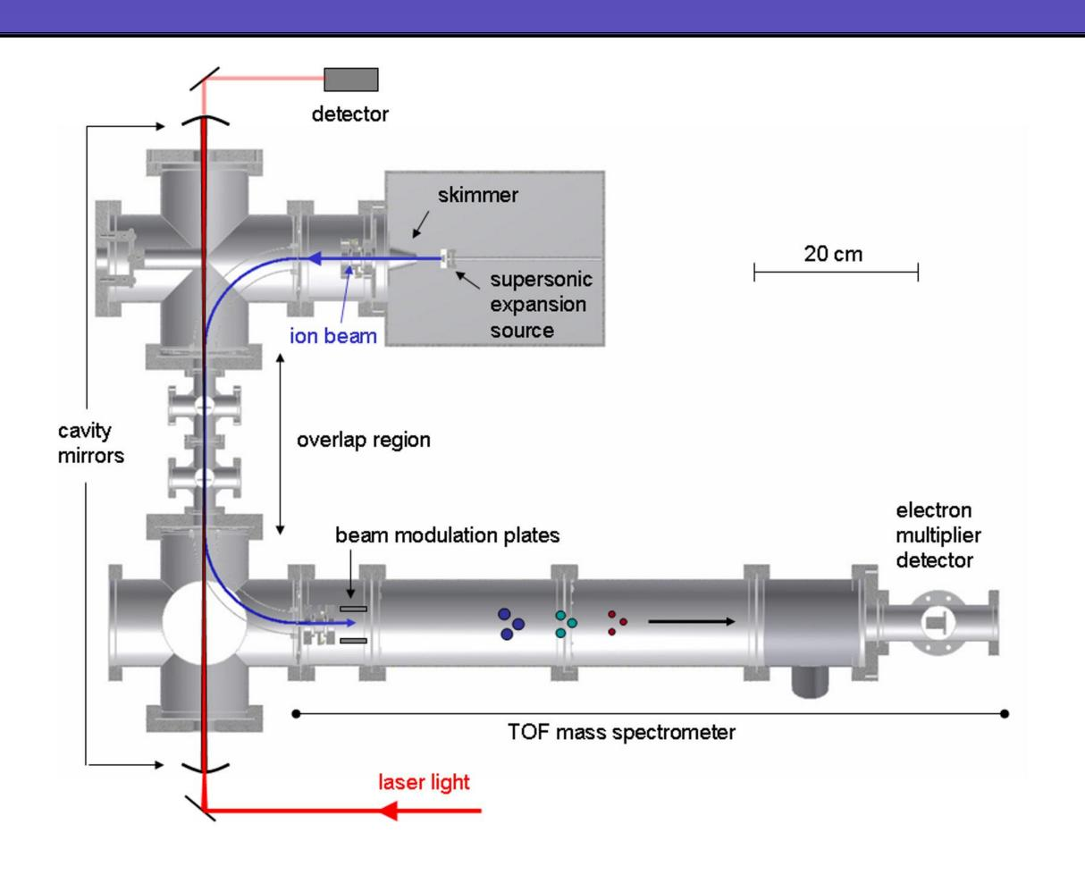
The McCall research group is interested in obtaining high resolution gas-phase spectra of astronomically important ions at astrophysically relevant temperatures. In order to accomplish this, our group has been developing an instrument called SCRIBES (Sensitive Cooled Resolved Ion BEam Spectroscopy). This technique combines a supersonic expansion discharge source with sensitive laser spectroscopy, and mass spectrometry.
