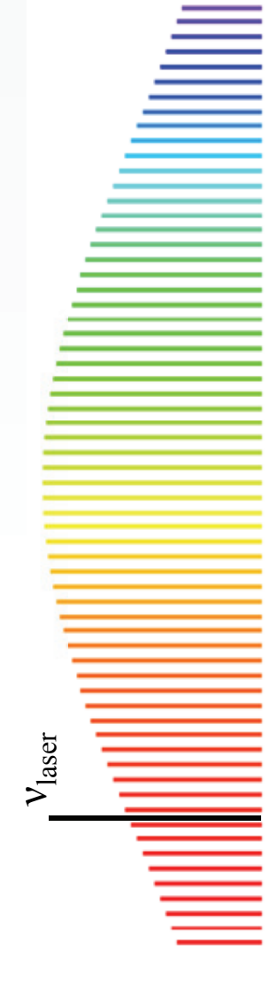
Conceptual diagram of the frequency comb. Frequency calibration is a result of the beat note from the cavity.
