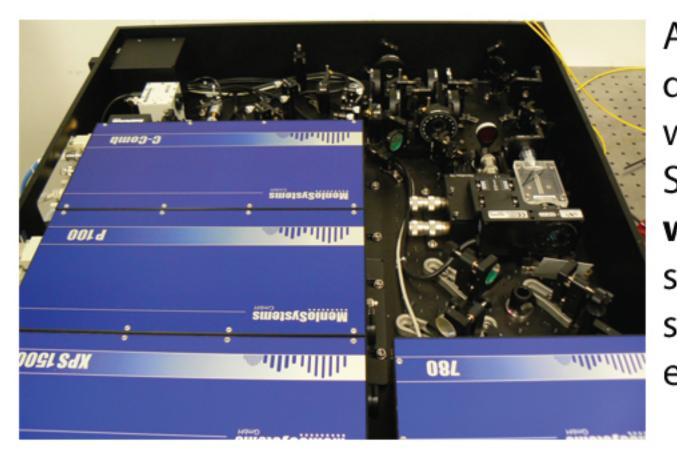
A continuous supersonic expansion discharge source can be interfaced with the SCRIBES experiment. SCRIBES promises **narrow linewidths** due to kinematic compression, facilitating the acquistion of spectra with the **high precision** necessary for performing combination differences analyses.
