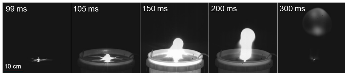
Figure 2. A series of images obtained using the Phantom v5.2 high-speed camera from a single plasmoid discharge with the ring as the cathode. A scale bar is included. The video corresponding to these images is included in the Supplemental Materials.
