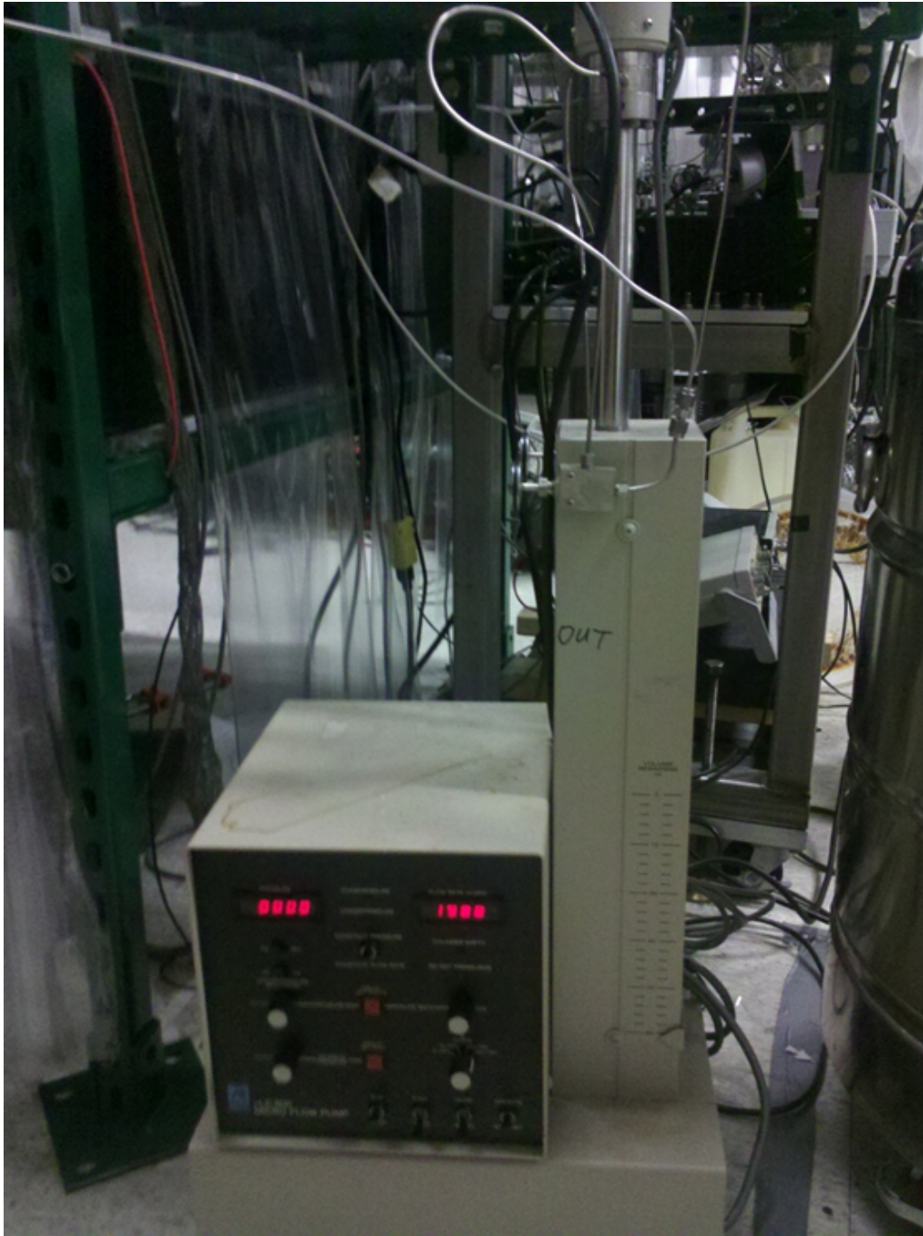
Figure 4.3: High-pressure syringe pump. Both the first- and second-generation sources used the same ISCO uL500 high-pressure syringe pump. The pump is capable of reaching pressures well in excess of those used in the source.
